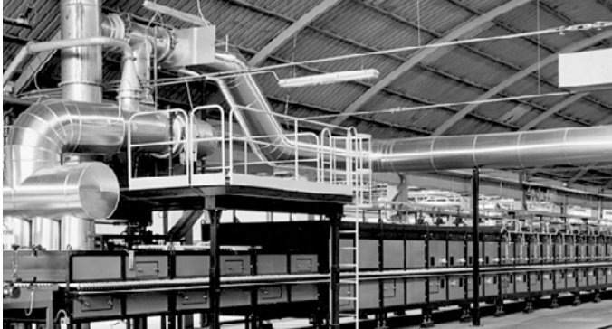
Roller hearth kiln in the ceramics industry
